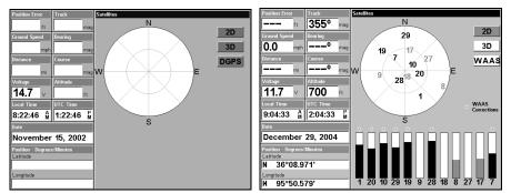
Satellite Status Page. Left view indicates unit has not locked on to any satellites and does not have a fix on its position. Right view shows satellite lock-on with a 3D position acquired (latitude, longitude and altitude), and WAAS reception.
